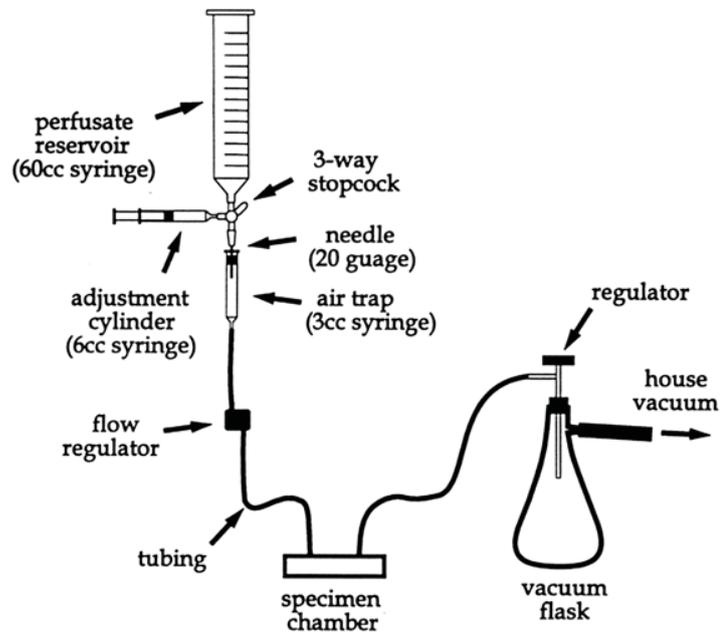
Fig. 19.3 – Schematic diagram of a simple perfusion system for maintaining tissue slices on the microscope stage. The gravity perfusion system is constructed using readily available syringes, three-way stopcocks, and tubing. The perfusion rate is adjusted using a simple thumb-wheel regulator. Perfusate is removed through a vacuum line and flask.
